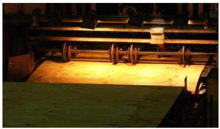
The ribbon of veneer passes from the lathe through manual or automated clipping machines which cut or 'clip' the veneer to size, or into smaller strips if defective material has been removed. In some mills producing high quality thin veneer, clipping is done after the continuous ribbons of veneer have been dried so as to maximise the number of full sheets obtained.
